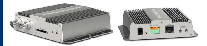
The NVS102 Network Video Server digitizes analog video and then transmits the signal across an IP network - such as a LAN, Intranet or Internet. This allows you to take your first step in implementing an IP-based system without having to install new network cameras. Besides, the loop-out analog video also enables connection to existing CCTV equipment such as DVR, etc.
